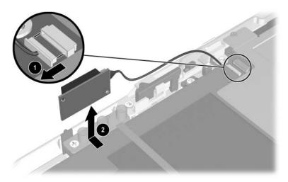
Removing the Bluetooth Wireless Module
